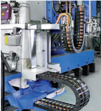
Plastic cable carriers on a roll neck milling machine.
